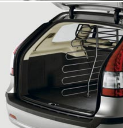
Cargo guard – metal guard that separates the passenger and luggage compartments. (Accessory, SportCombi only.)
